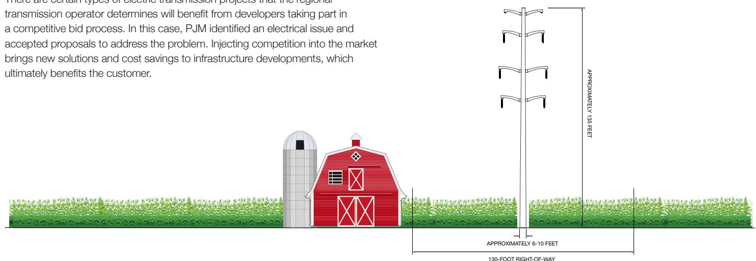
The rendering depicts a typical 230 kV double-circuit steel monopole; however, engineering standards or topography may require a variance in structure type or height along the route.
